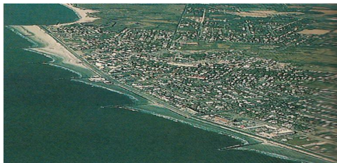
Photo 6. Beach filling process between jetties (in the given case between the capes)
